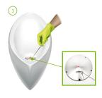
Swipe the flag of the uridan logo with the magnetic pen. The LED light should light up red to indicate if there is no uriLOCK in the urinal. If the LED lights up green, the waste trap requires more water.
