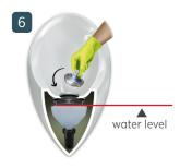
Fill the water to the point of overflow and insert the cover.
